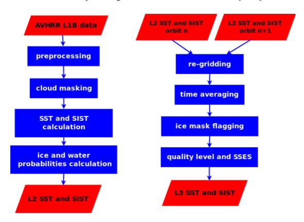
Figure 2: NHL OSI SAF Sea and Ice Surface Temperature L2 and L3 processing chains overview.
